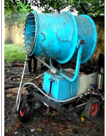
Picture 3: Trolley Mounted Mist Canon at JK Nagar Railway Siding
